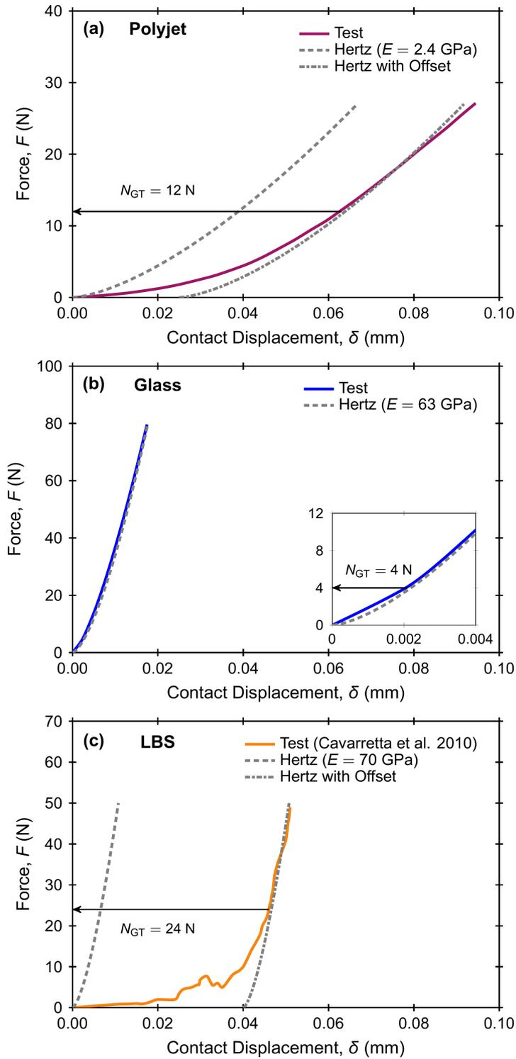
Figure 4: Uniaxial particle-particle compression test results on (a) polyjet 3D printed and (b) glass equal-sized spheres (after Ahmed and Martinez 2020), and (c) single grain crushing test result on Leighton Buzzard Sand (LBS) (after Cavarretta et al. 2010). Note: diameter of the spheres is 3.175 mm, and the diameter of the LBS particle is 1.67 mm
